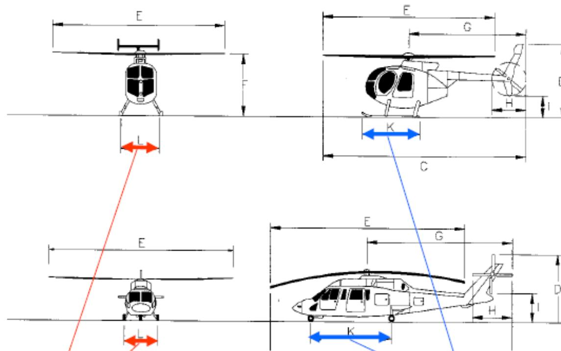
**UC = Maximum width or length of the undercarriage:** used to define some characteristics.
