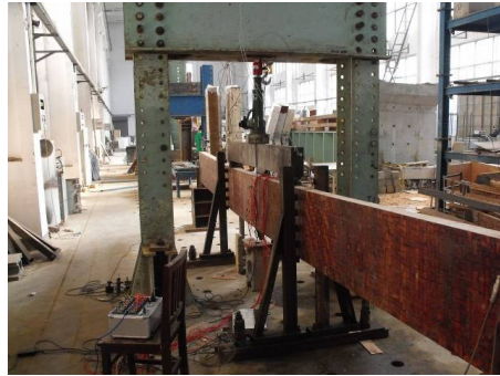
Fig. 12 Fatigue test of full-scale glubam girder
