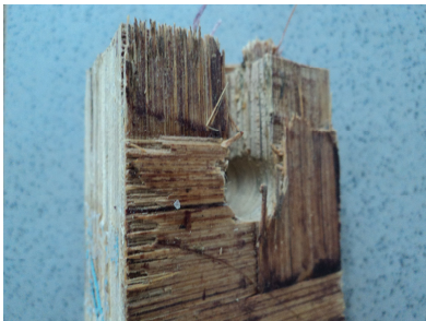
Fig. 8 Failure mode of V group-shearing out
