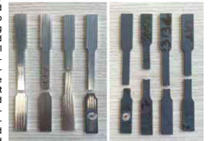
Politecnico di Milano, March 2016. Cold Spray Inconel 718 samples after tensile test, pre heat-treatment (left) and post heat-treatment type A (right).
