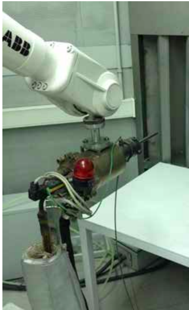
CPT - Universitat de Barcelona, May 2016. Spraying system used to deposit the amorphous metal thick coatings.
